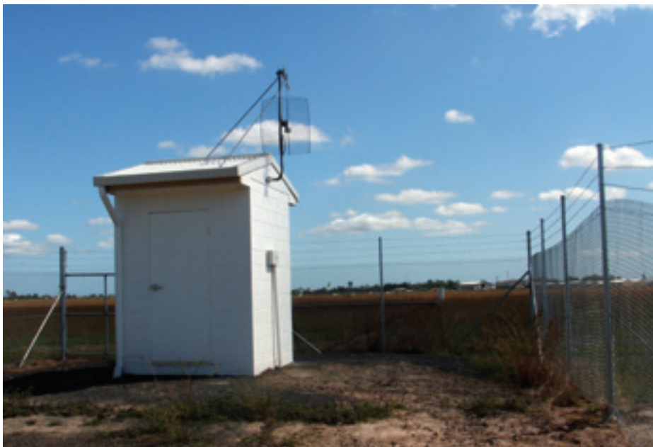
The Trimble NetR5 GPS station
